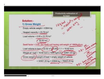
So, let us see how to proceed with this problem. So, the first thing you have to estimate is your gross weight of the machine. So, your gross weight of the machine is nothing but your empty weight plus the weight of the load in the machine, weight of the load in this scraper bowl. So, this is your gross weight the empty weight is given by the manufacturer. Now, I need to find what is the weight of the load in the machine?
