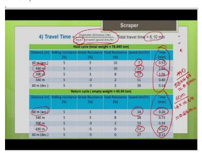
So, now, you need to calculate the travel time. So, we have calculated the speed. You know the speed for different segments. You know the haul distance for different segments. Now, you can calculate the travel time. So, time is nothing but your distance by speed, for every segment you are going to calculate it. Say for the first 60 meter, the speed is given in kilometers per hour 7 kilometer per hour. Haul distances is in meter.
