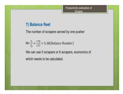
Now let us see the balanced number of scrapers which are served by one pusher. So, that is equal to n is nothing but number of scrapers served by one pusher. It is equal to cycle time of the scraper by cycle time of the pusher. So, here we have estimated the cycle time of the scraper as 7.78 minute. And the pusher cycle time is 1.37 minutes. So, it is 7.78 divided by 1.37 gives you the value as 5.68.
