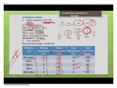
So, now the next step is we have to determine what are all the resistance in the haul route? The rolling resistance is uniform throughout the haul route. Is given in the question is 50 kg per ton or equivalent gradient as 5%. So, whatever way you express, you can take it accordingly. Then the grade resistance, the grade resistance is given for different sections, which we discussed just now. For the first 500 meters it is +5%.
