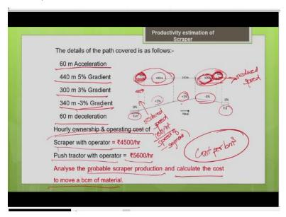
The other input data given is about the path about the haul route, about the haul distance and the resistance encountered in the haul route. So, we can see this is a pictorial representation of the haul route. You have the cutting area, you have the fill area, this is your haul route. So, you can see that for the first initial 500 meters, it is upslope, you have a gradient of +5%.
