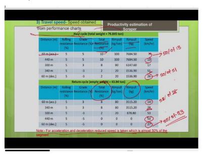
Now I need to determine the travel speed from the performance chart. The total weight of the machine is express in tons 1000 kg equal to 1 ton. Accordingly, we have to convert it into tons. So, during the haul cycle, it is a loaded condition 76.845 ton. During return cycle it is empty. So, the empty weight of the vehicle is 43.94 tons. So, you have already calculated your total resistance already in both percentage as well as kg per ton. We are already determined in the earlier slide.
