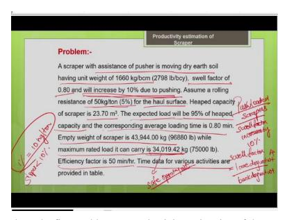
So, now, let us work on the first problem on productivity estimation of the scraper. So, a scraper with the assistance of the pusher is moving the dry earth soil having unit weight of 1660 kg per bank meter cube. So, you can see that this is a conventional pusher loaded scraper, here we are moving the material which is dry earth soil, its unit weight is given 1660 kg per bank meter cube.
